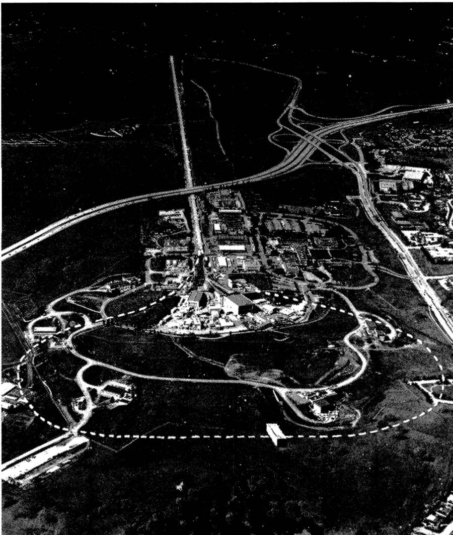
The new Stanford Linear Collider — after acceleration in the two-mile linac, the electron and positron beams are brought together to collide (once only) in the experimental hall in the foreground.
